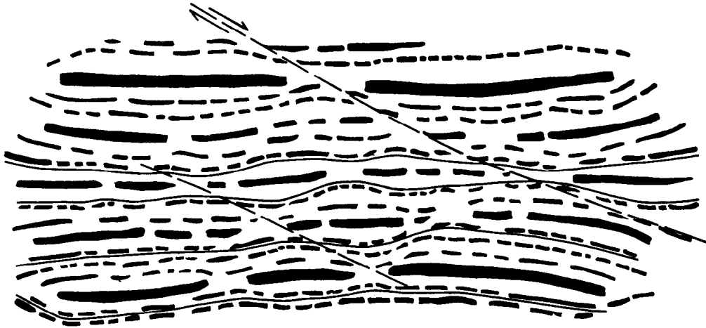
Fig. 9. Line drawing of Fig. 7, showing the spatial relationship between the rectangular boudins in the thick competent layers (dark), the large scale pinch-and-swallow instabilities indicated by the solid lines and the conjugate normal kink bands indicated by the dashed lines.
